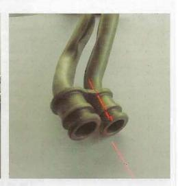
on-contact tube measurement has been well known in the international tube market ever since Homer Eaton introduced the first Laservision Measuring table from Eaton Leonard in 1973. Since then the non-contact fork has set a high standard for tube measurement.
