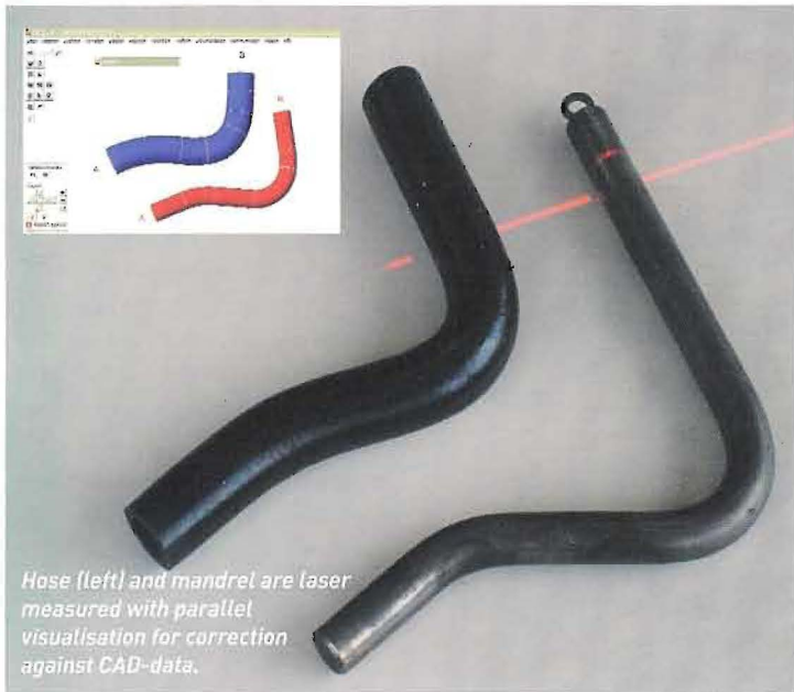
Freeform bend-measured tube with complete data sets for correction against CAD and bender.
