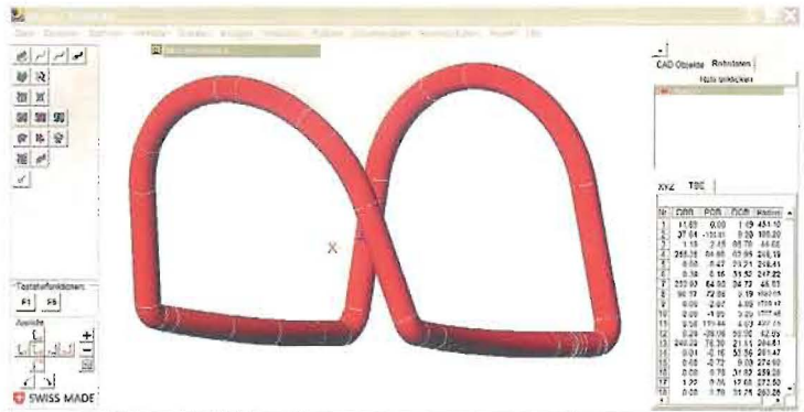
Freeform bend-measured tube with complete data sets for correction against CAD and bender.
